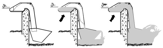
No flow until water level reaches elevation  $\mathbf{H}_{\mathbf{a}}$ .
